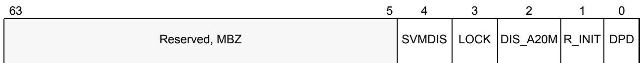
Figure 15-15. Layout of VM_CR MSR (C001_0114h)
