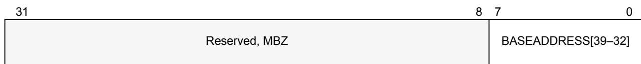
Figure 15-9. Format of DEV_BASE_HI[n] Registers
