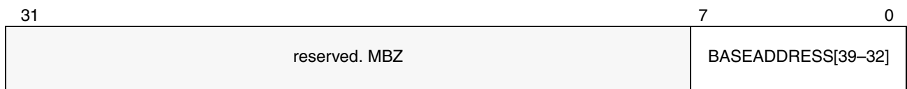
Figure 15-9. Format of DEV_BASE_HI[n] Registers
