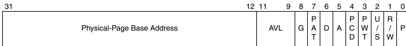
Figure 5-6. 4-Kbyte PTE—Non-PAE Paging Legacy-Mode
