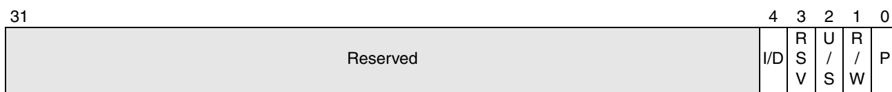
Figure 8-3. Page-Fault Error Code
