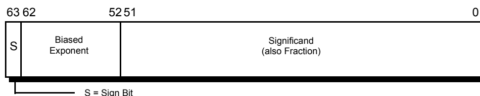
Figure 4-4. Floating-Point Data Types
