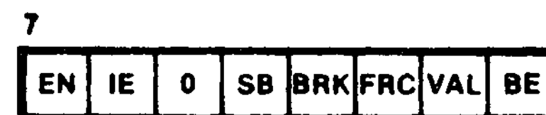
Figure 9-15. Transmitter Control/Status Register
