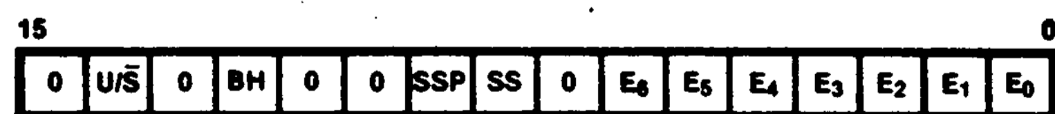
Figure 3-5. Master Status Register
