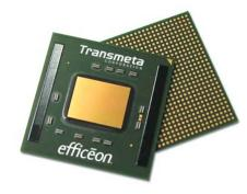
DRAM, a 1.6 GB/s HyperTransport™ interconnect, and an AGP 4X graphics interface. With the new Code Morphing Software for the Efficeon processor, Transmeta extends its leadership in power management, offering a solution that provides high performance while consuming less power for the same work. The result is a highly efficient x86 solution suitable for notebook computers, Tablet PC's and many other applications where an integrated, low power x86 processor is desirable.
