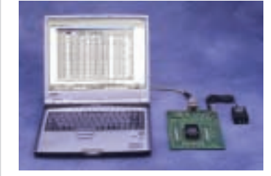
Connection example * The user is required to connect write signals and mount oscillators as appropriate to each device.
