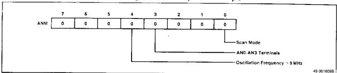
Figure 8-7. Setup of A/D Channel Mode Register for ADC Operation Example
