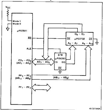
Figure 4-16. Setup of Memory Mapping Register for ROM Part Memory Expansion Example
