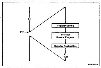
Figure 9-6. Flowchart 2: Interrupt Processing Sequence
