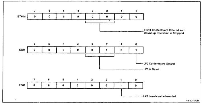
Figure 6-19. Specifying PC<sub>6</sub> for CO<sub>0</sub> Output in Programmable Waveform Output Example
