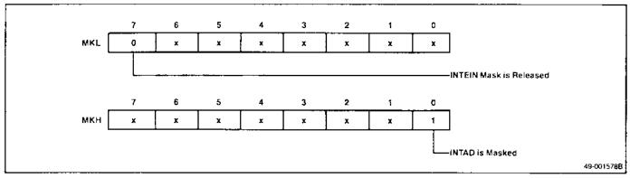
Figure 6-25. Setup of ETMM for Initialization Phase of Single-Pulse Output Example
