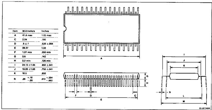
Figure C-2. 64-Pin Plastic Shrink DIP (750 mll)
