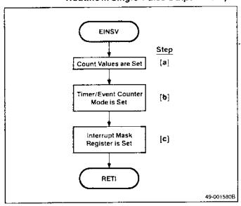
Figure 6-27. Setup of ETMM and EOM for INTEIN Interrupt Phase of Single-Pulse Output Example
