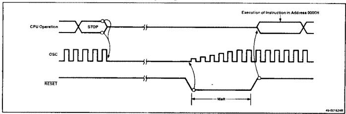
Figure 10-8. Software Stop Mode Release Timing
