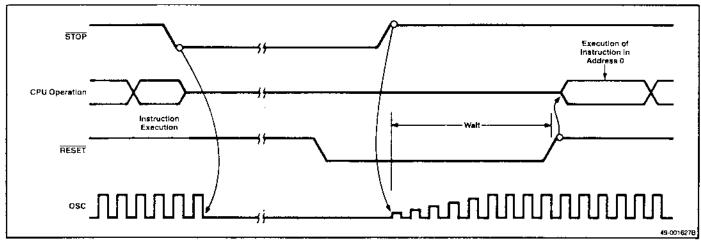
Figure 10-11. RESET After STOP Goes Low to High
