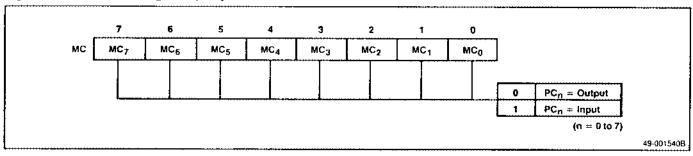
Figure 4-7. Mode Control C Register (MCC)
