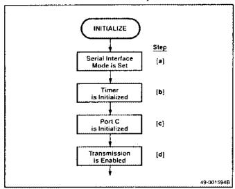
Figure 7-12. Setup of Serial Mode Registers for Initialization Phase of Serial Data Transfer Example
