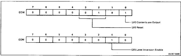
Figure 6-15. Example of Setting Up ETMM for Programmable Waveform Output on COo
