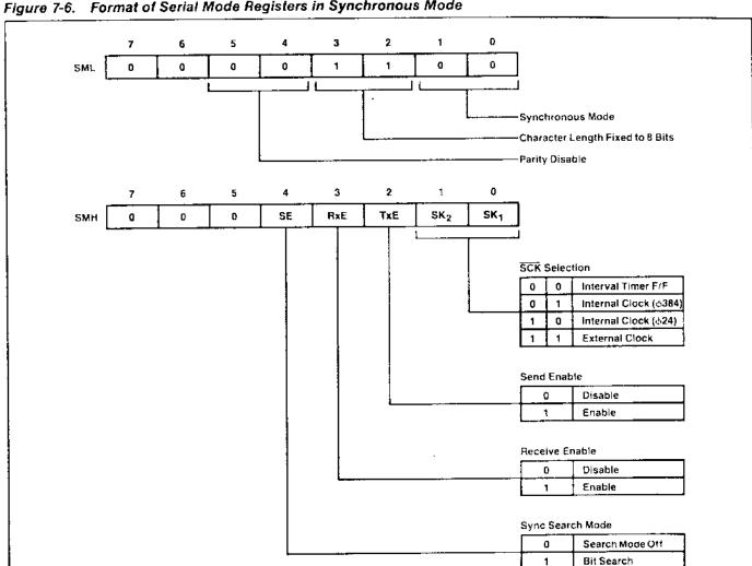
Figure 7-6. Format of Serial Mode Registers in Synchronous Mode
