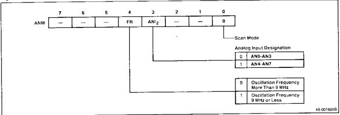
The conversion process is continued from either the ANO or AN4 input, independent of whether or not the interrupt is accepted, with new results stored in the respective conversion result registers. This will continue until the ANM register is modified. In this mode, up to four analog signals can be converted to digital form with a minimal amount of software.
