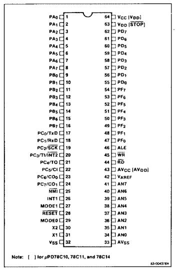
Figure 1-2. Pin Configuration, 64-Pin Plastic Miniflat
