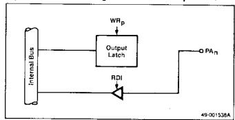
Figure 4-2. Mode A Register (MA)
