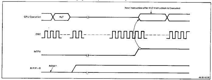
Figure 10-4. Standby Mode for 7810, 7810H, 7811, and 7811H
