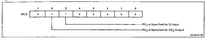
Figure 6-24. Setup of Interrupt Mask Register for Initialization Phase of Single-Pulse Output Example
