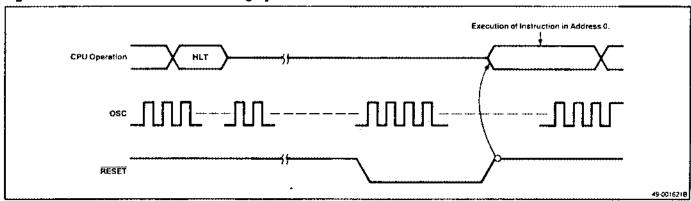
Figure 10-2. Half Mode Release Timing by Interrupt With Interrupts Enabled
