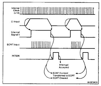
Figure 6-12. Setting Up ETMM for Pulse-Width Measurement Operation
