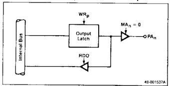
Figure 4-4. Block Diagram of a Port A Input Line
