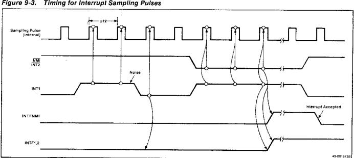
Figure 9-3. Timing for Interrupt Sampling Pulses
