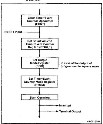
Figure 6-6. Setting Up ETMM for Interval Timer Operation
