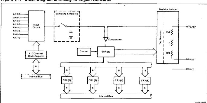
Figure 8-1. Block Diagram of Analog-to-Digital Converter
