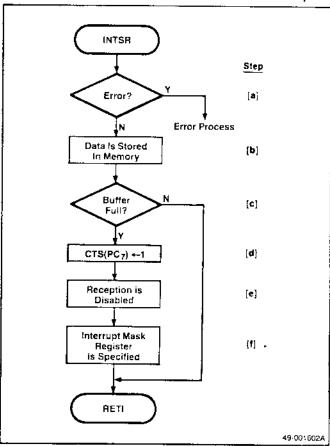
Figure 7-18. Setup of Interrupt Mask Register in Receive-Enable Phase of Serial Data Transfer Example
