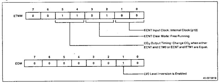
Figure 6-28. Setup of Interrupt Mask Register for INTEIN Interrupt Phase of Single-Pulse Output Example
