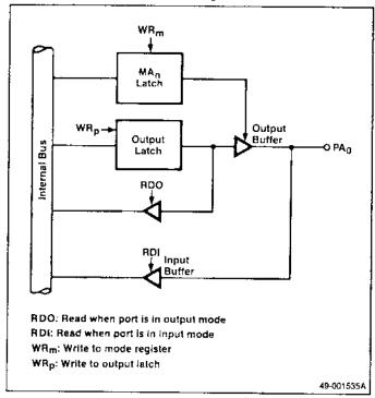
After reset, the contents of the port A output latches are undefined.
