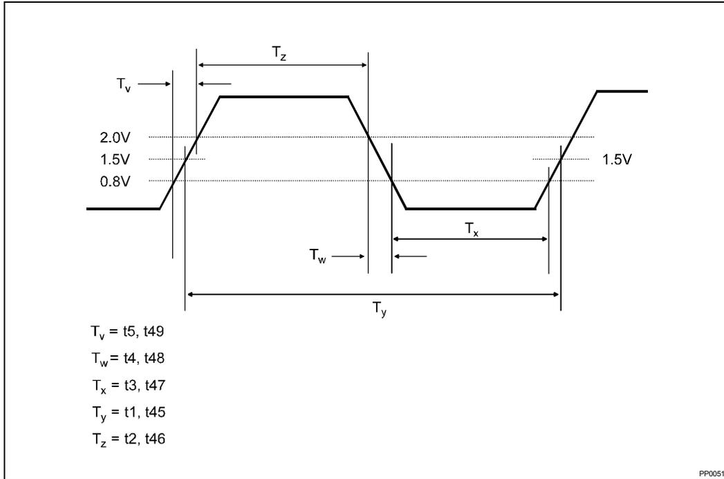
Figure 3. Clock Waveform
