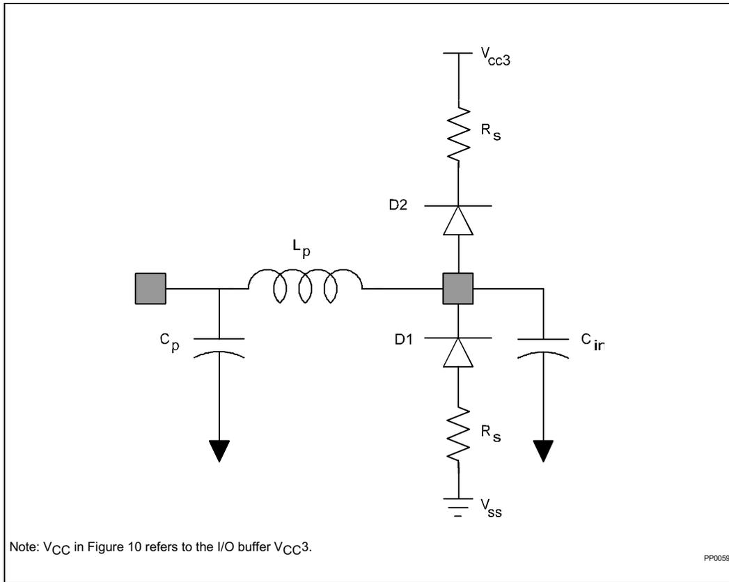
Figure 10. Input Buffer Model, Except Special Group
