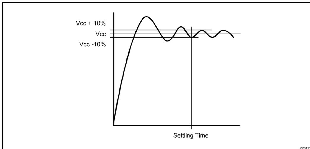
Figure 14. Settling Time
