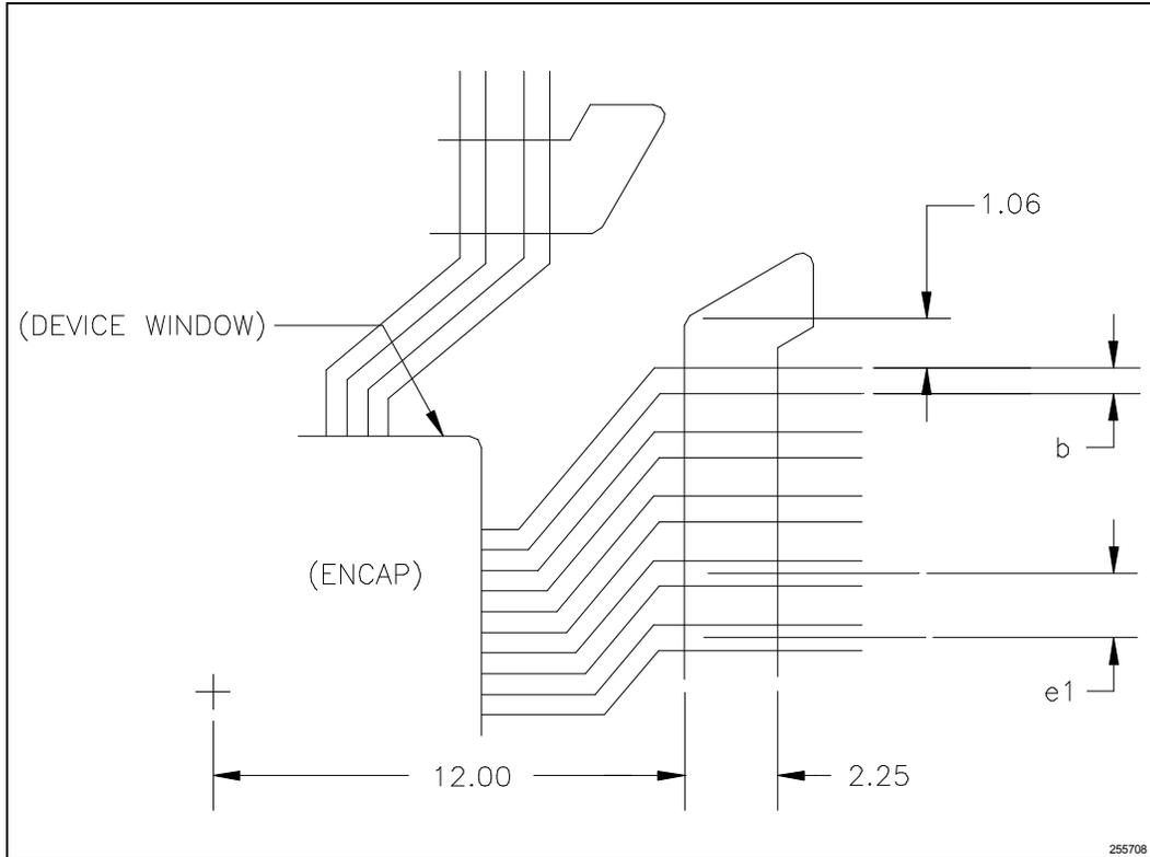
Figure 19. Outer Lead Bond (OLB) Window Detail
