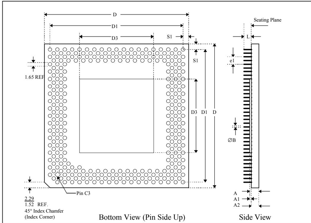
Figure 22. 296-Pin Ceramic Pin Grid Array Package
