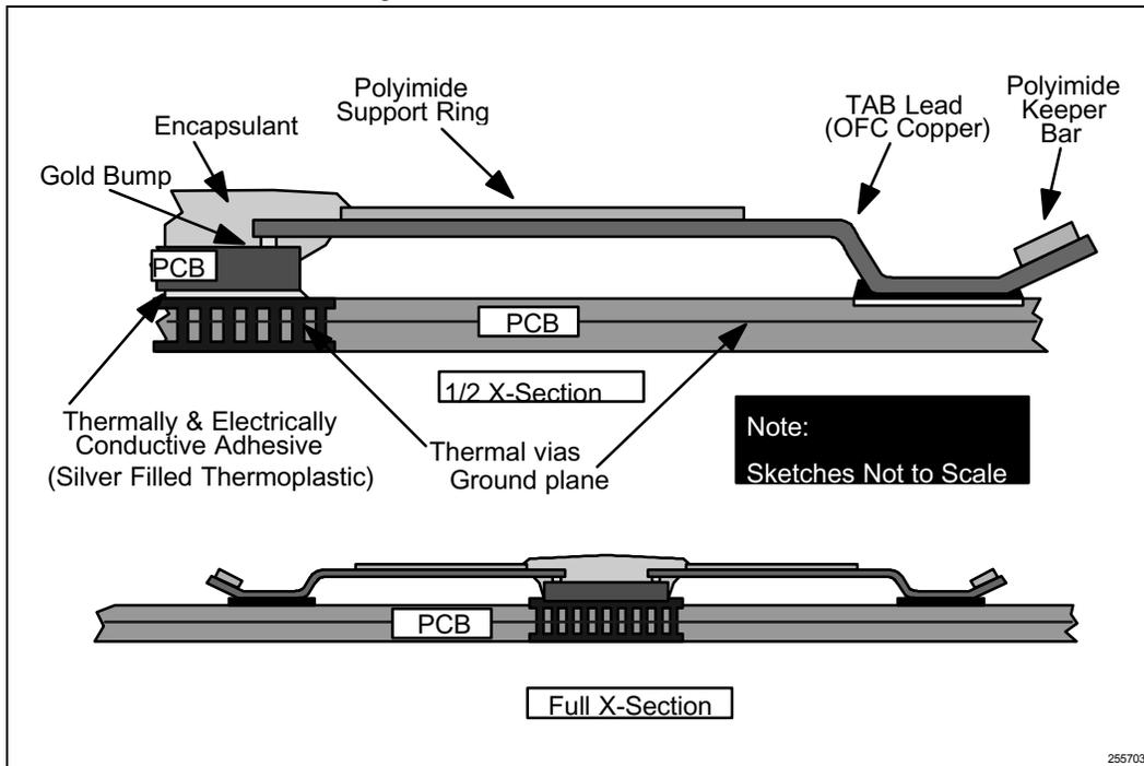
Figure 15. Cross-Sectional View of the Mounted TCP
