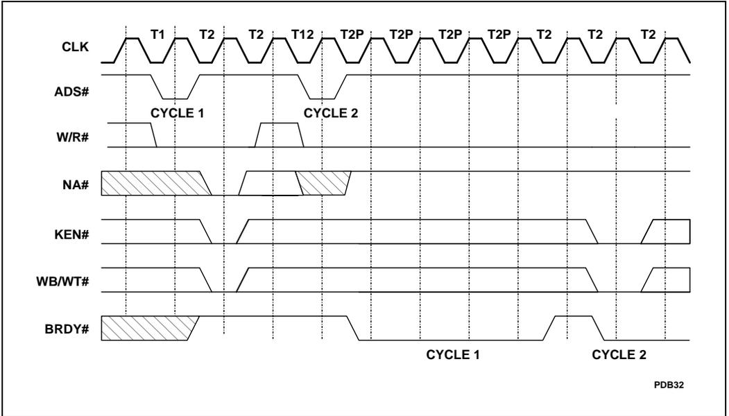
Figure 6-20. KEN# and WB/WT# Sampling with BRDY#
