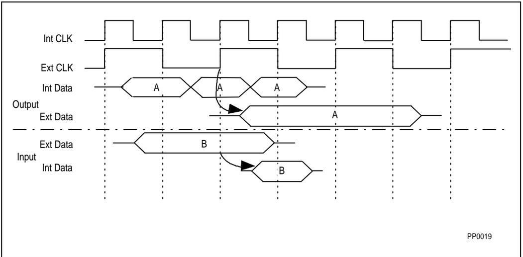
**Figure 19-2. Pentium® Processor (610\75, 735\90, 815\100, 1000\120, 1110\133) 1/2 Bus Internal/External Data Movement**
