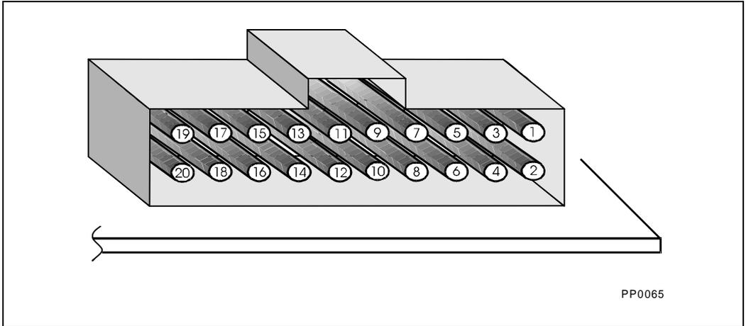
Figure 31-1. Debug Port Connector
