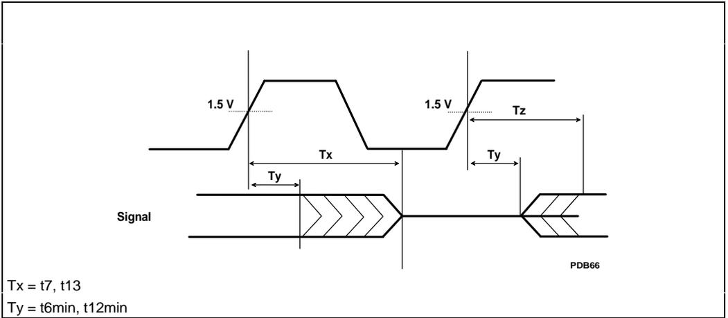
Figure 7-3. Float Delay Timings
