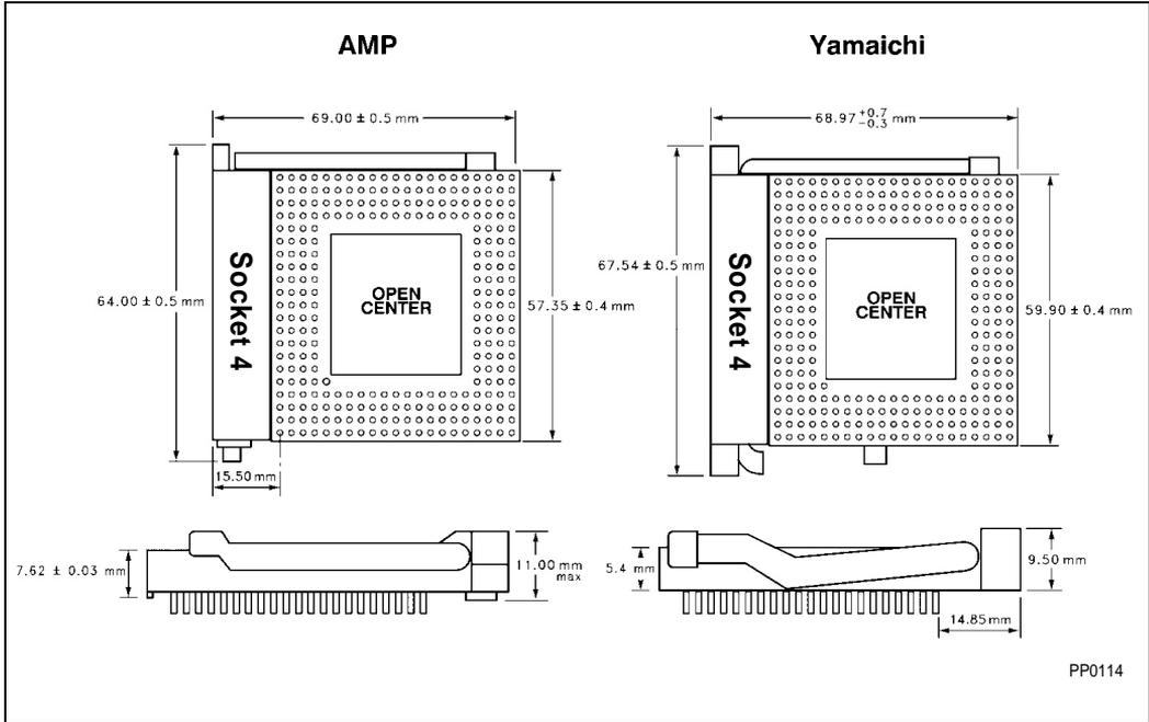
**Figure 16-1. Socket 4 Footprint Dimensions**
