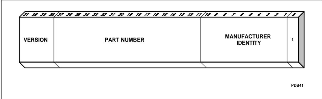
**Figure 11-3. Format of the Device ID Register**
