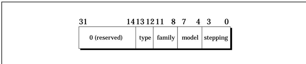
**Figure 20-1. EAX Bit Assignments for CPUID**
