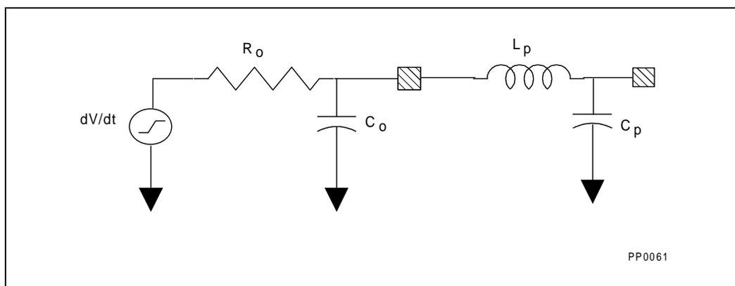
**Figure 24-3. First Order Output Buffer Model**
