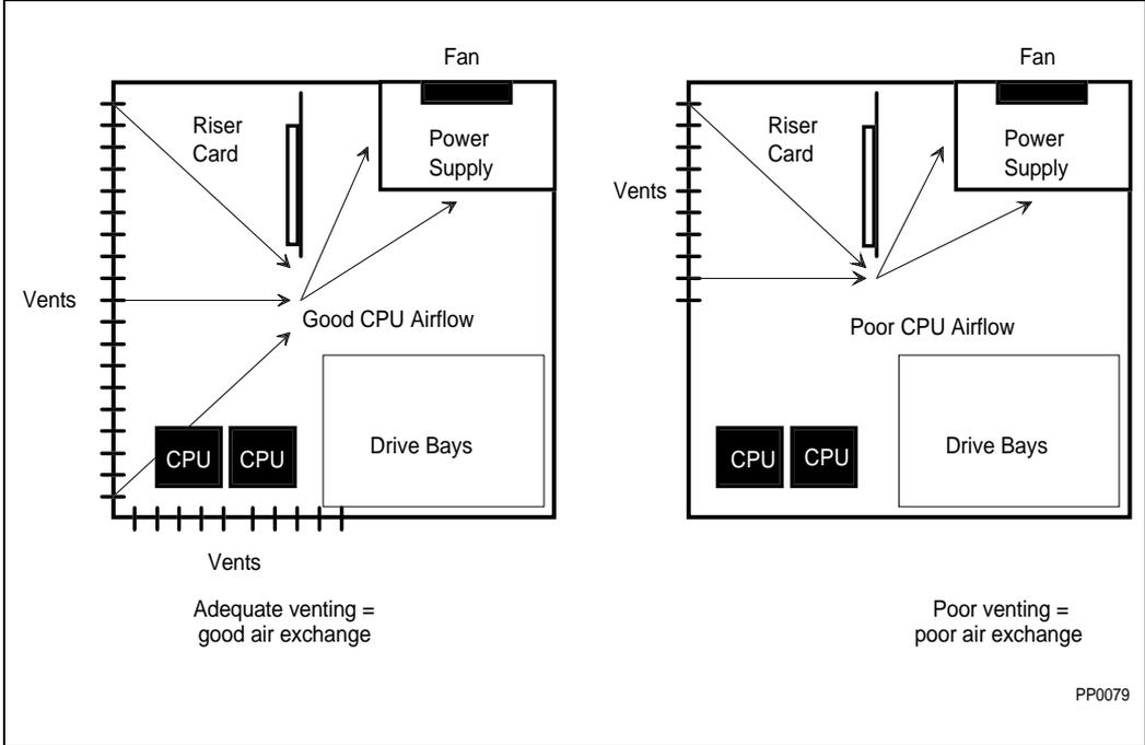
**Figure 32-5. Examples of Air Exchange Through PC Chassis**
