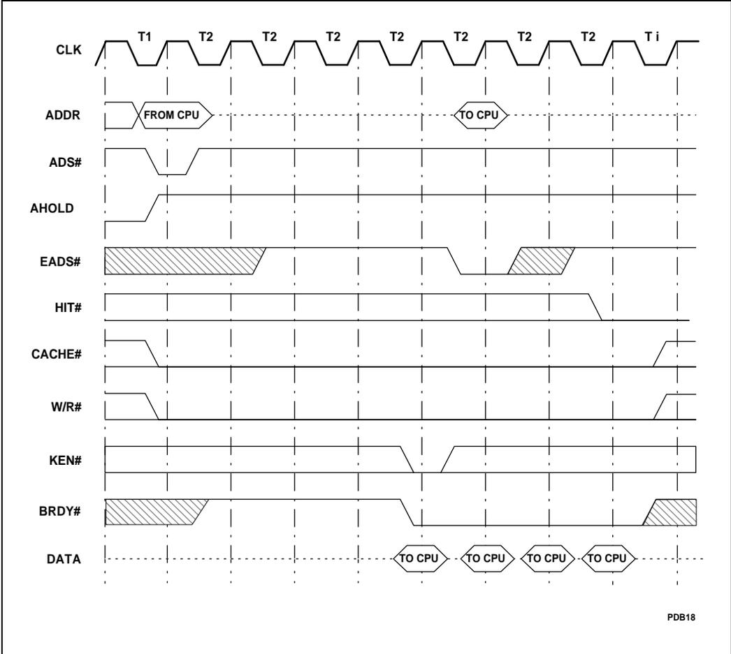
Figure 6-26. Snoop Responsibility Pickup — Non-Pipelined Cycles
