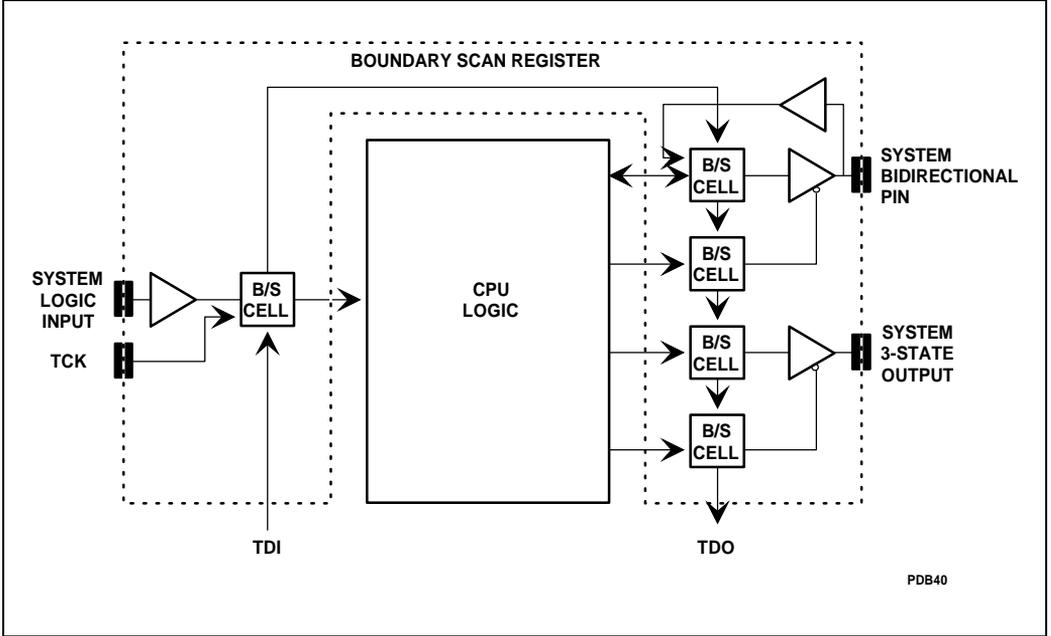
Figure 11-2. Boundary Scan Register
