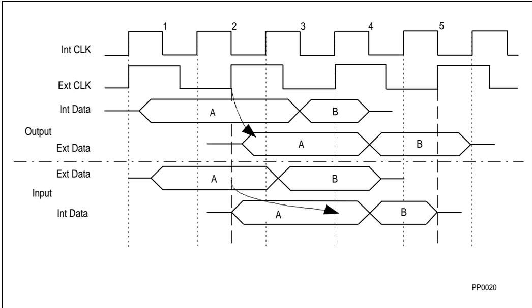
**Figure 19-3. Pentium® Processor (610\75, 735\90, 815\100, 1000\120, 1110\133) 2/3 Bus Internal/External Data Movement**
