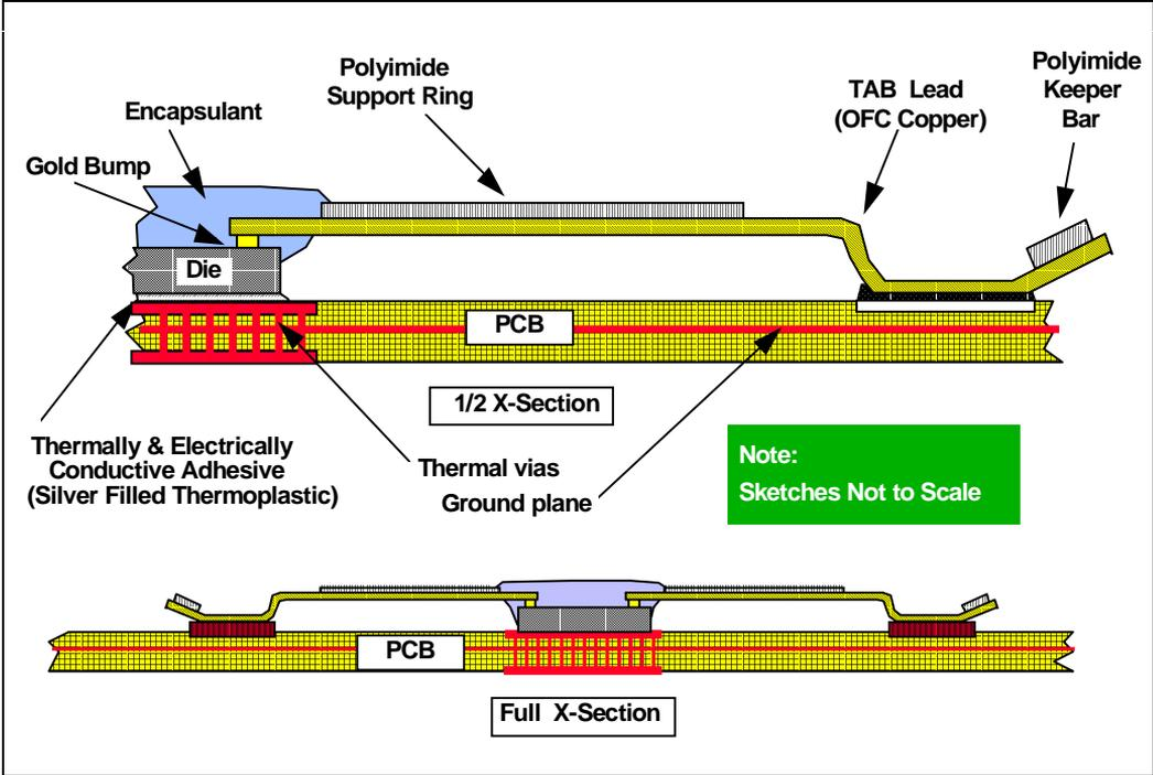
Figure 34-2. Cross-Sectional View of the Mounted TCP Package
