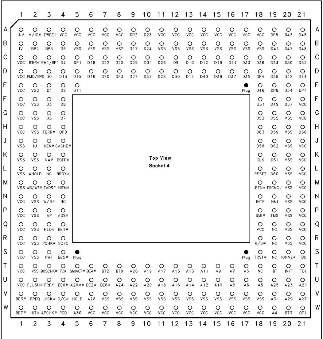
Figure 16-3. Socket 4 Pinout (Top View)
