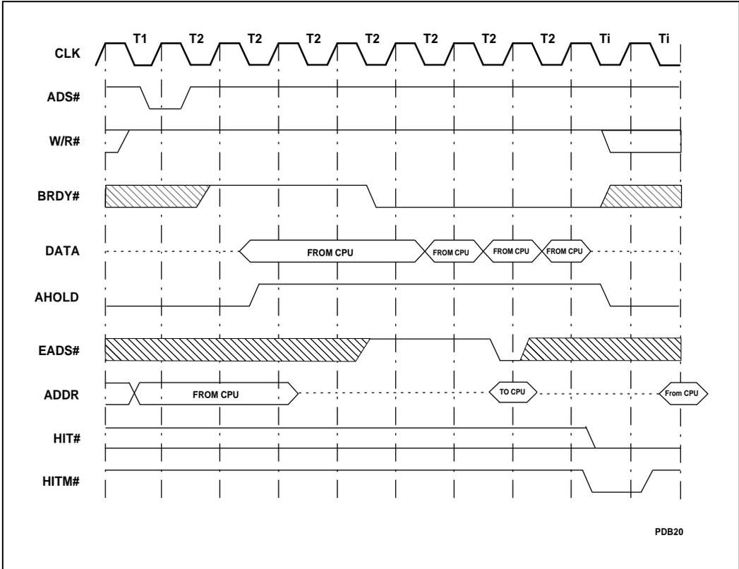
Figure 6-28. Latest Snooping of Writeback Buffer
