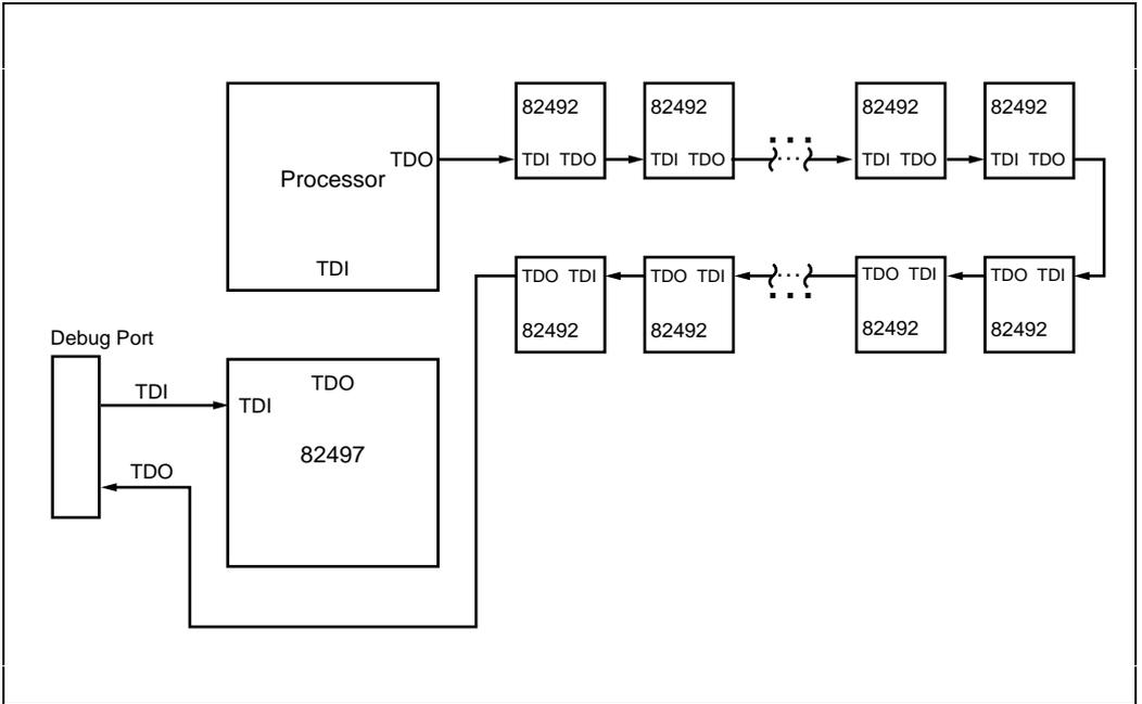
Figure 31-7. Example of Multiple Components in Scan Chain
