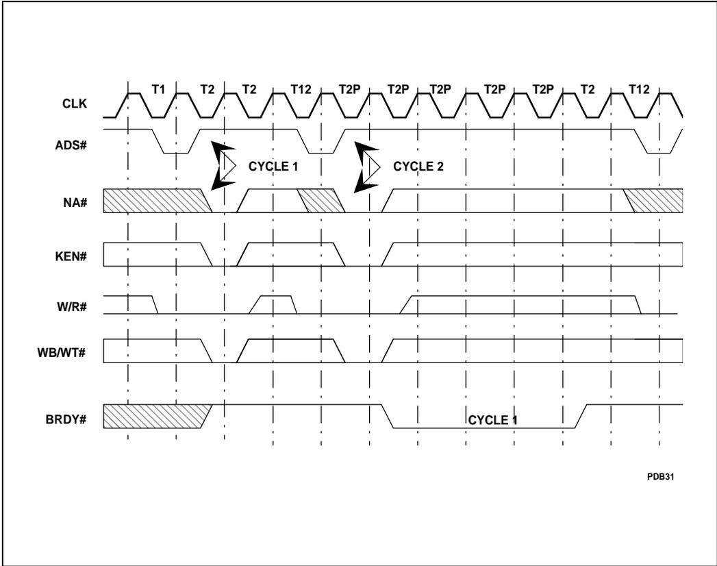
Figure 6-19. KEN# and WB/WT# Sampling with NA#
