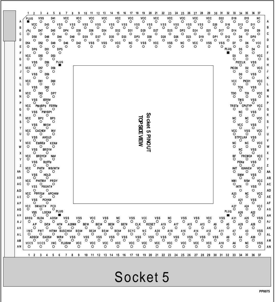
Figure 32-1. Socket 5 Pinout — Top Side View
