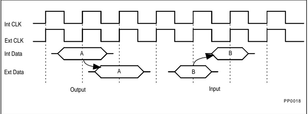
**Figure 19-1. Pentium® Processor (510\60, 567\66) Synchronous Internal/External Data Movement**
