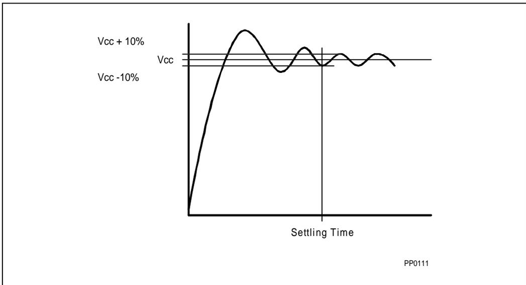
Figure 24-5. Settling Time
