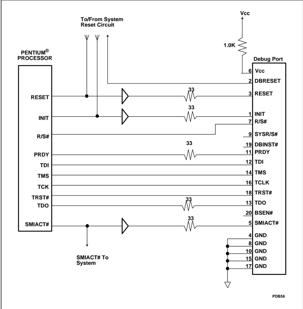
Figure 15-2. Minimal Debug Port Implementation
