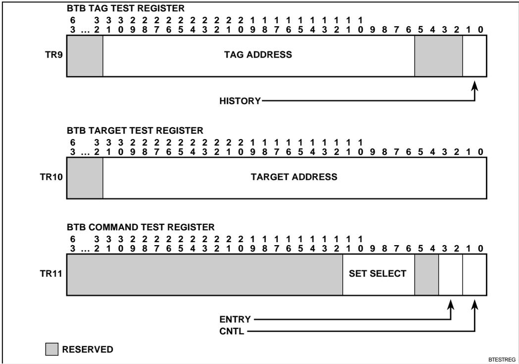
Figure 33-3. BTB Test Registers
