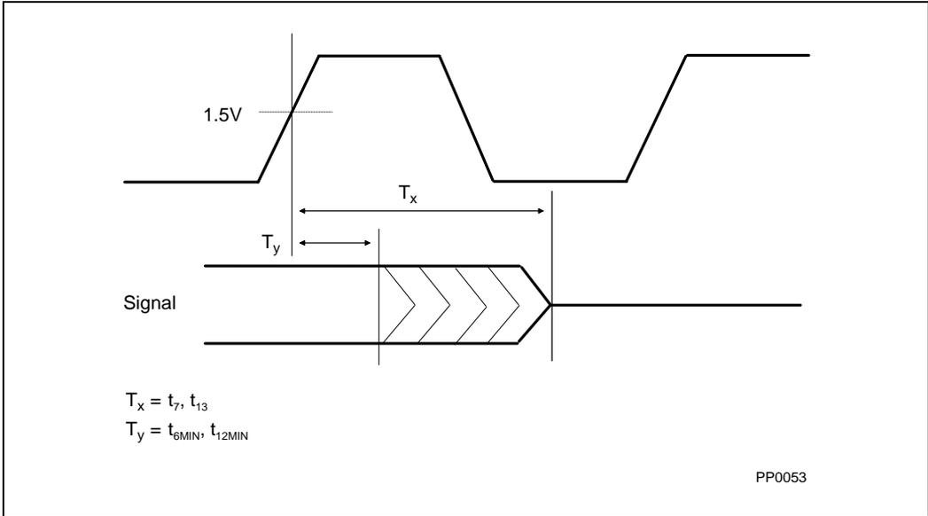
Figure 23-3. Float Delay Timings
