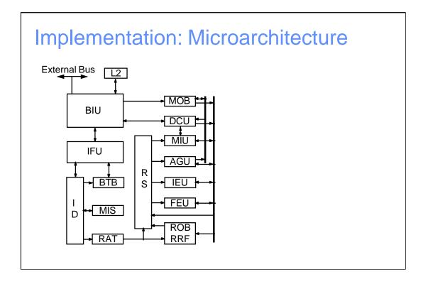
Let's take a look at the block diagram of the P6 processor to see how it fundamentally works. The processor is organized in three sections:
