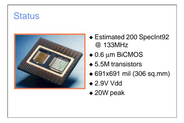
The first thing to notice is that there is something different about the first P6 processor: there are actually two die in the package. The one on the left is the L2 cache. The one on the right is the CPU. These die are wire bonded into the same package allowing a full speed interface to the L2.
