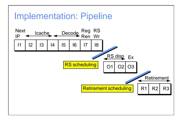
So now you've seen the basic way that the machine flows, and the way micro-ops flow through the machine. It may have occurred to you that there seems to be a lot of work going on in here, so how deeply pipelined must this machine be?
