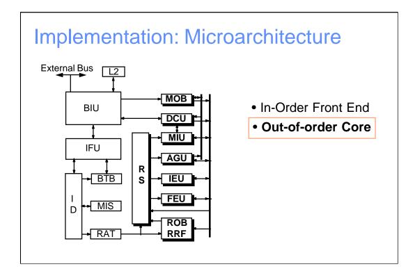
The other place is the reorder buffer. It determines which micro-ops at any given moment are capable of being retired. They are capable of being retired only if they have actually executed, they have all the results ready, it is their turn in line and there is no other thing pending. We will return to retirement momentarily, but the important thing is that when the micro-op has actually executed, the results go back to the reorder buffer so that the ROB knows that it is completed.
