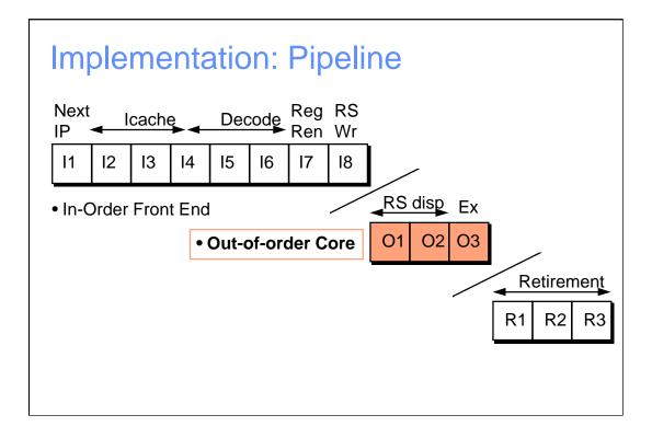
Processor Pipeline: Out-of-Order Core
