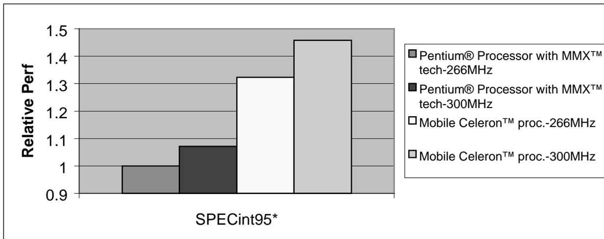
Figure 1. Mobile Celeron™ Processor Relative Performance for SPECint95
