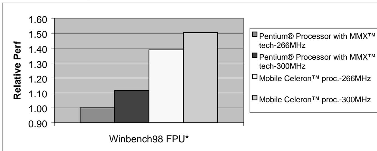
Figure 5. Mobile Celeron™ Processor Relative Performance for Winbench98 FPU\*
