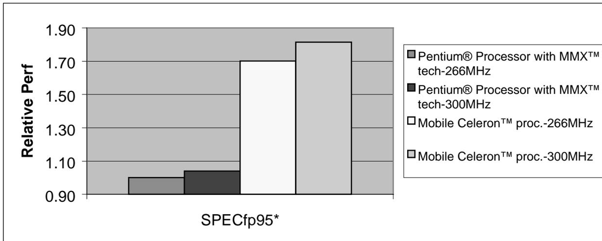
Figure 4. Mobile Celeron™ Processor Relative Performance for SPECfp\*95
