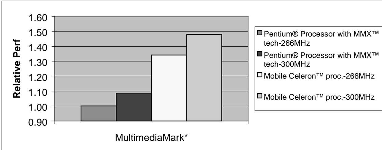
Figure 3. Mobile Celeron™ Processor Relative Performance for MultimediaMark\* 99 Benchmark
