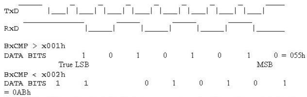
False LSB = Extra bit clocked in internally causing the false MSB to = 7th data bit, not the 8th.
