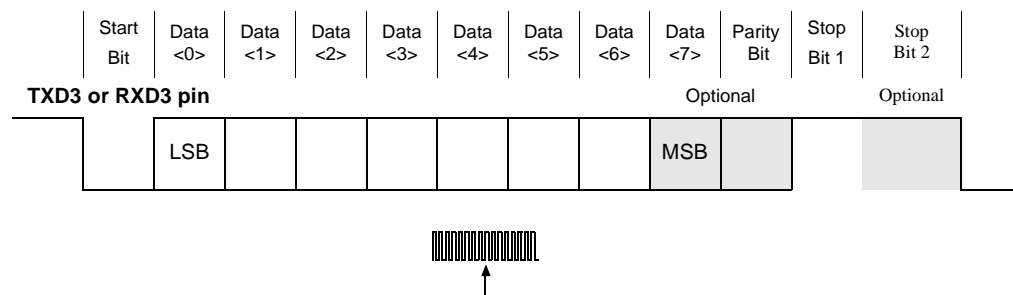
Figure 11-29. Example UART Data Frame
