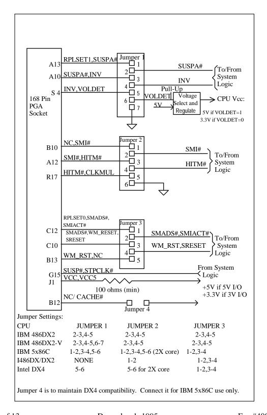
The following Common Socket Schematic illustrates a method of using jumpers to enable a common PGA socket to service any of the listed processors.
