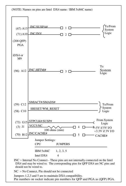
Socket specification shows how a design can accommodate several different 486 bus microprocessors.
