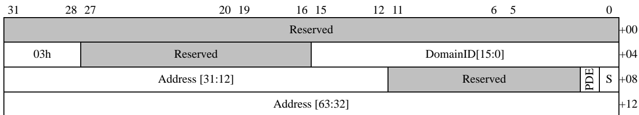
Figure 15: INVALIDATE_IOMMU_PAGES Command Encoding
