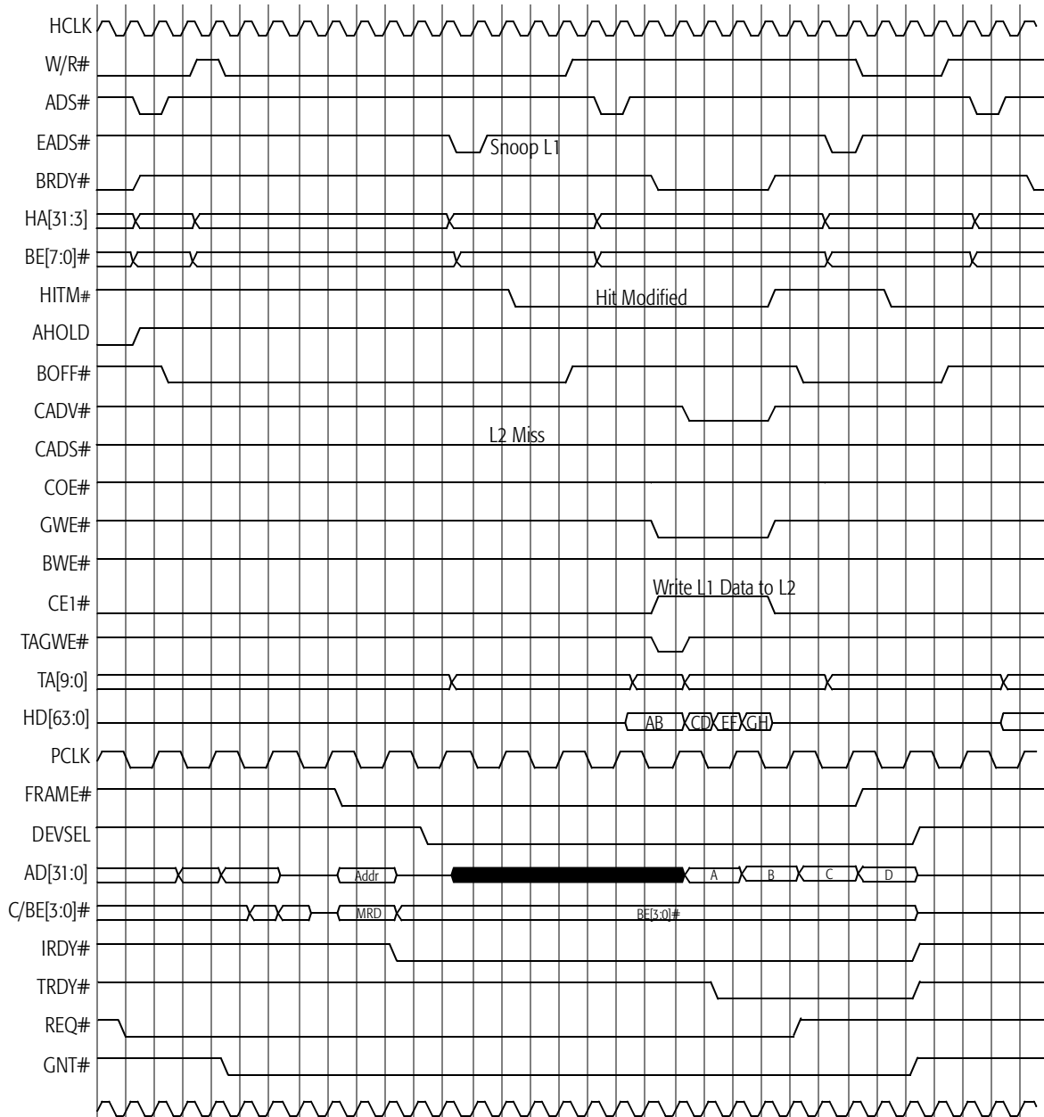
Figure 5-27. PCI Bus Initiator Read: Modified L1 Hit
