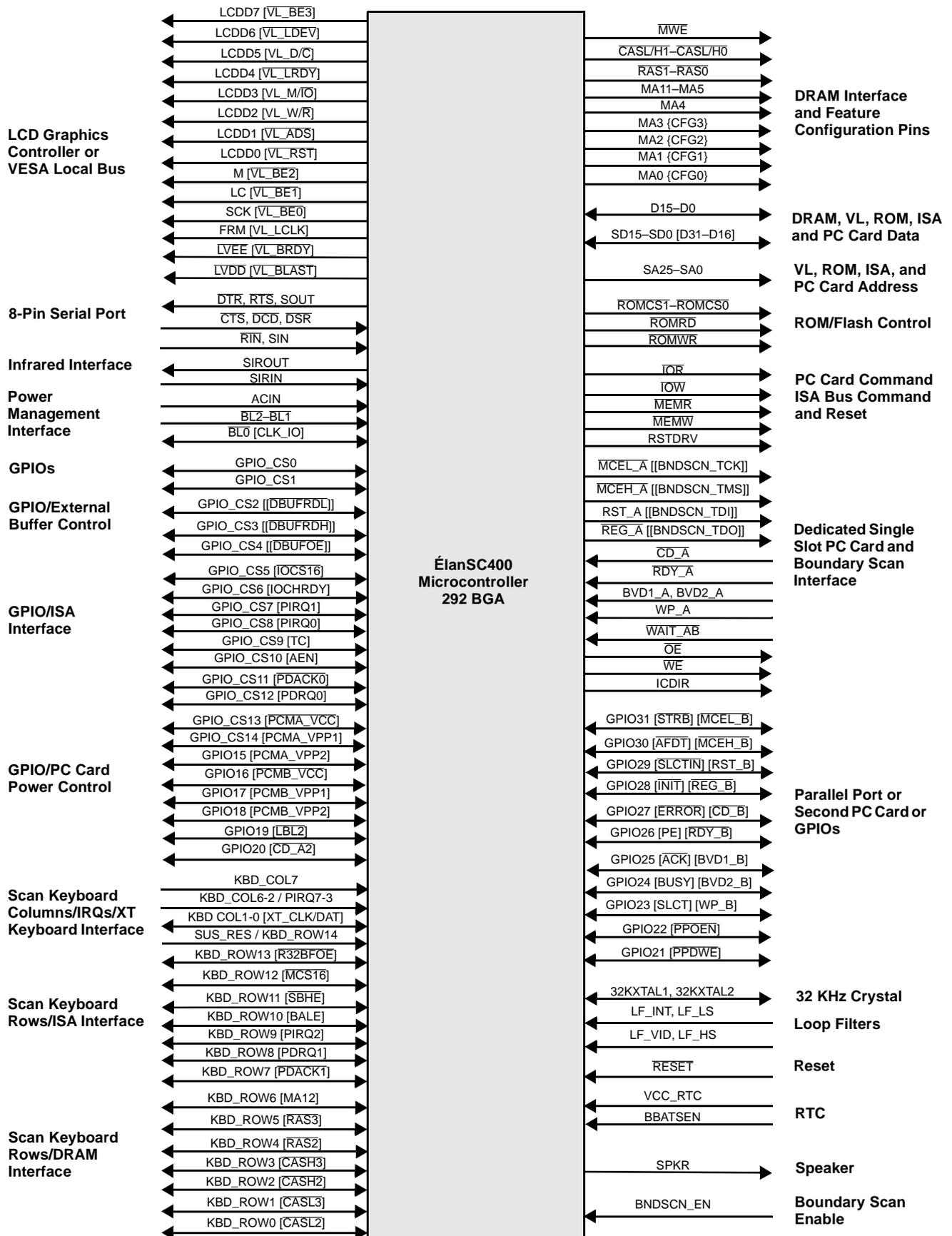
**Note:** / = Two functions available on the pin at the same time. { } = Function during hardware reset. [ ] = Alternative function selected by firmware configuration. [[ ]] = Alternate function selected by a hardware configuration pin state at power-on reset.
