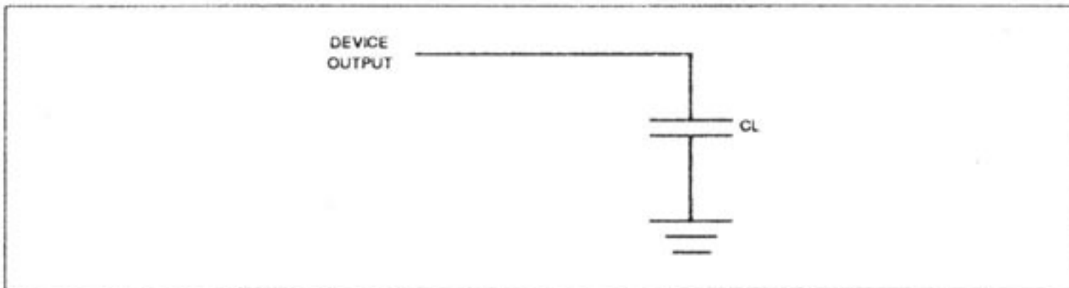
AC Test Loading on Outputs
