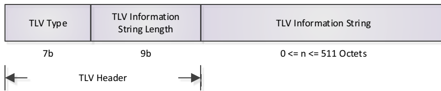
Figure A-11. Structure of an LLDP TLV
