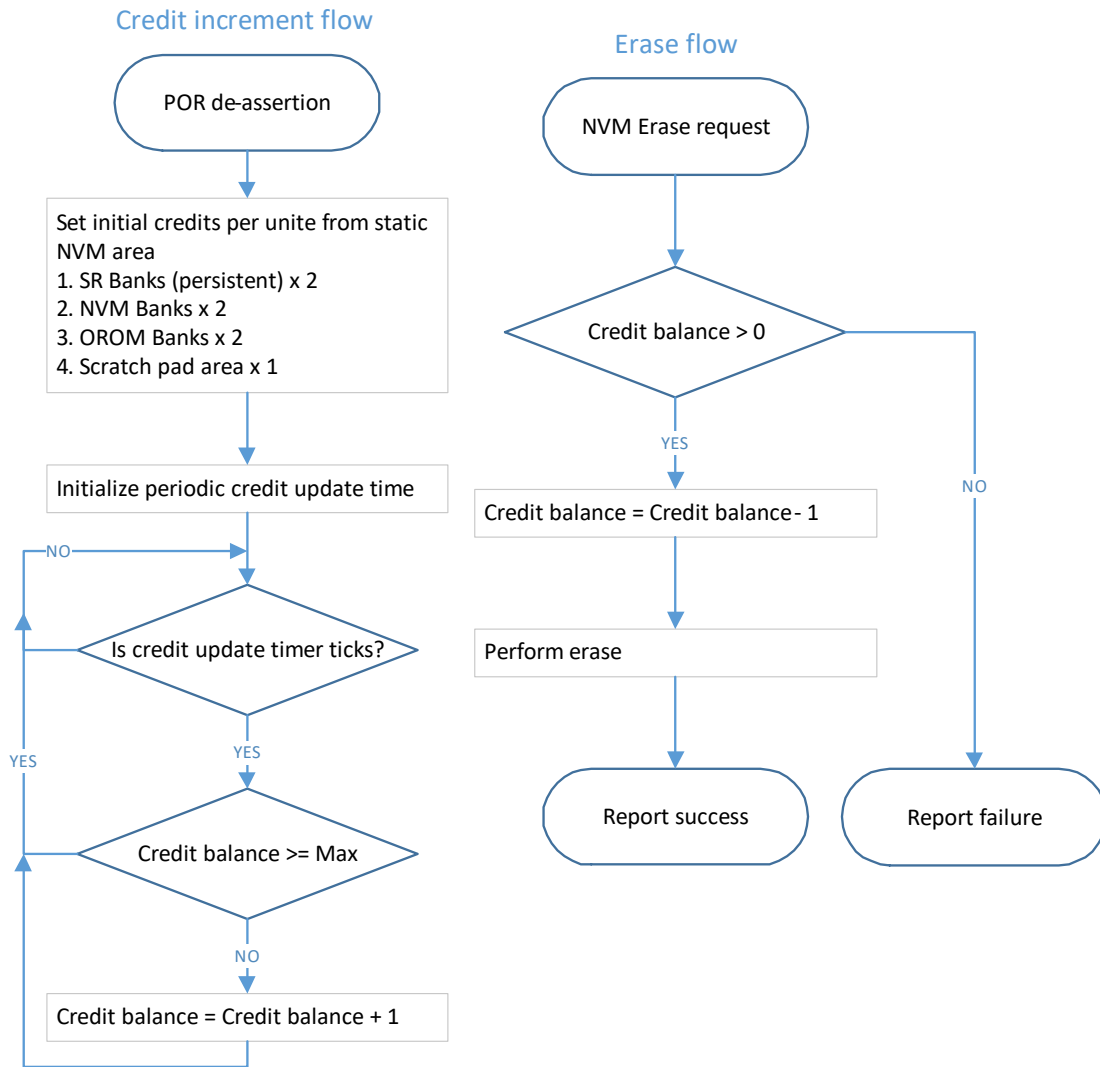
Figure 3-33. Flash Wear-Out Protection Algorithm 1
