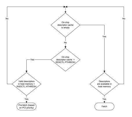
Figure 3-3. Receive Descriptor Fetching Algorithm
