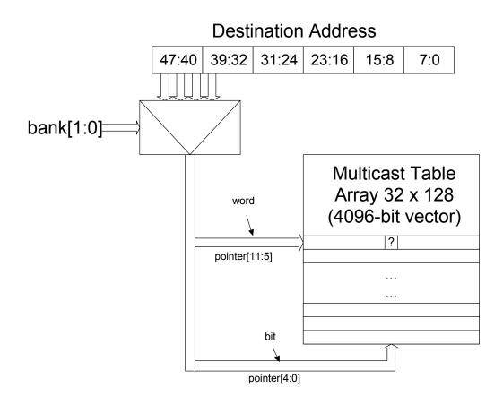
Figure 13-1. Multicast Table Array
