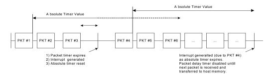
Case C: Packet timer expiring while a packet is transferred to host memory. Illustrates that packet timer is re-started only after a packet is transferred to host memory.
