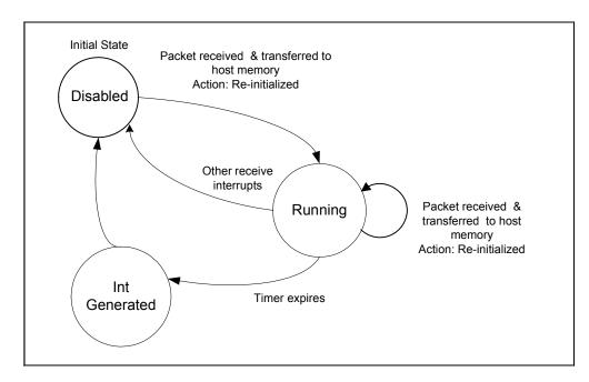
Figure 3-4. Packet Delay Timer Operation (State Diagram)
