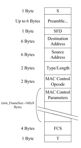
*Note:* "S" is the Start-of-Packet delimiter and "T" is the first part of the End-of-Packet delimiters for 802.3z encapsulation.
