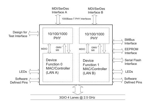
Figure 2-1. 82571EB/82572EI External Interface
