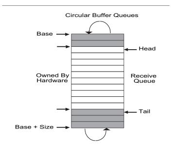
Figure 3-1. Receive Descriptor Ring Structure
