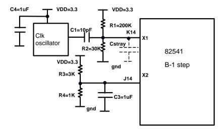
The oscillator solution for the 82541GI includes capacitor C1, which forms a capacitor divider with capacitor  $C_{\text{stray}}$  of approximately 20 pF. This attenuates the input clock amplitude and adjusts the oscillator load capacitance where
