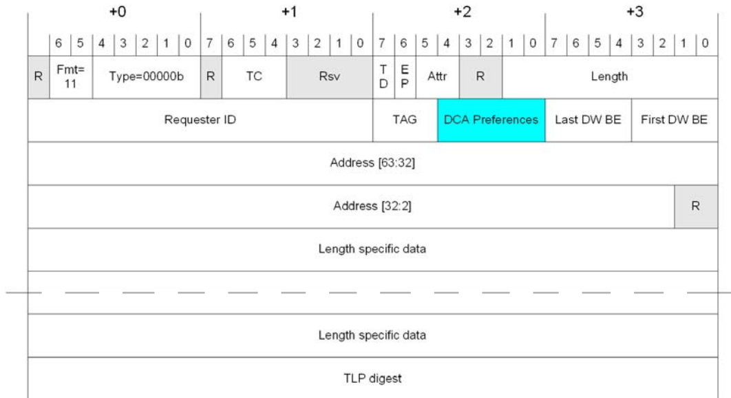
Figure 25. PCIe* Message Format for DCA
