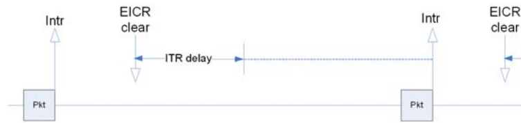
Figure 22. Case B: Light Load, Interrupts Immediately on Packet Receive
