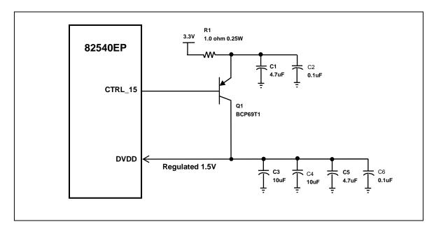
Note that the 82540EP also contains a "Maximum Power-Savings" mode to permit applications to reduce D3 no-wakeup power consumption. However, if "Maximum Power Savings" is utilized, then the on-chip LDO regulation circuits cannot be used, and power must be supplied via external voltage regulation.
