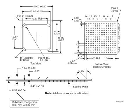
*Note:* No changes to existing soldering processes are needed for the 0.32 mm substrate change.
