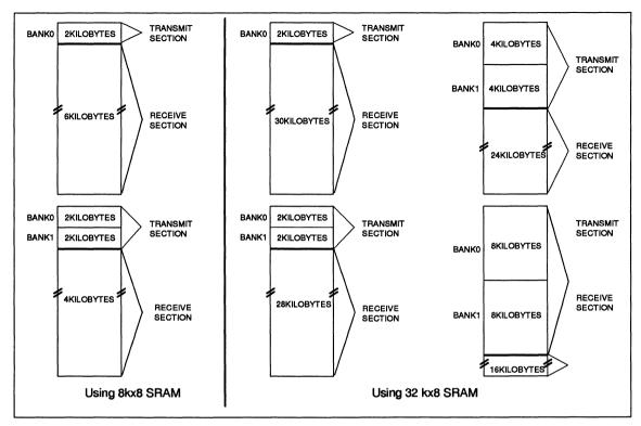
Figure 7. Transmit Buffer Configurations
