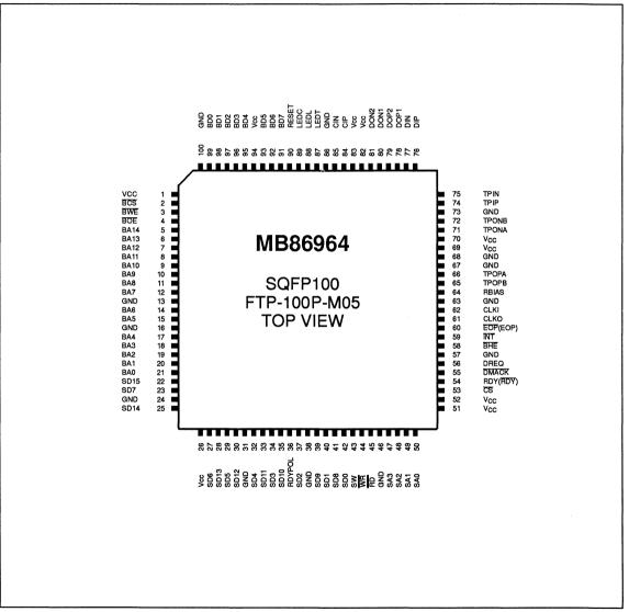
Figure 1. MB86964 Pin Assignments
