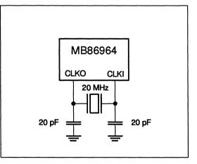
Figure 4. Crystal Oscillator Connection
