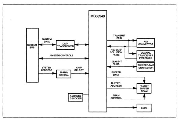
Figure 3. Typical Application, Block Diagram
