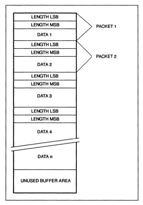
Figure 8. Transmit Buffer Detail
