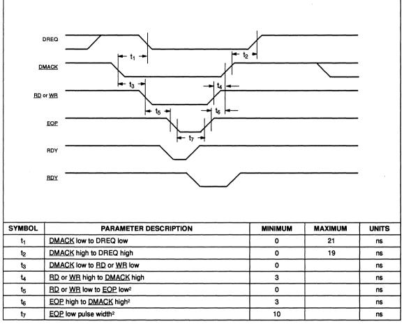
All of the <u>RD</u>, <u>WR</u> and <u>EOP</u> asserted pulses must fall inside of the <u>DMACK</u> asserted pulse. An asserted <u>EOP</u> terminates any further DREQ after <u>DMACK</u> returns high. The DMA cycle uses <u>DMACK</u> as the chip select. <u>DMACK</u> overrides SA<3:0>, torcing selection of the buffer memory port in a DMA cycle.
