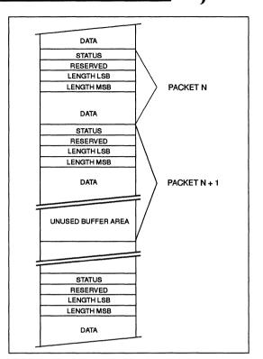
Figure 9. Receive Buffer Detail
