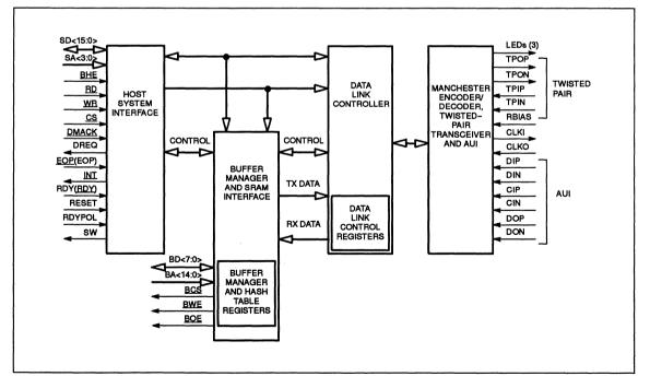
Figure 2. MB86964 Block Diagram
