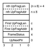
The first dword in the UPD is the UpNextPtr entry, which contains the physical UpNextPtr address of the next UPD in the uplist. If this is the last UPD in the uplist, then this value is zero.
