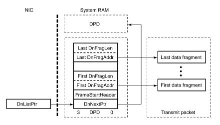
The driver places packets to be transmitted in data fragments (buffers) in system memory and then creates the list of DPDs that point to the fragments in system memory. All pointers are physical memory addresses (not virtual memory addresses).
