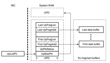
The head of the uplist is the UPD that corresponds to the current upload packet. The UpListPtr register points to this UPD. As the UPD is processed, the NIC fetches fragment address and fragment length values one at a time from the UPD and places them into NIC registers, which control the data upload operations.
