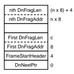
DPD length ranges from 16 to 512 bytes. Each DPD describes up to 63 fragments, which consist of pairs of DnFragAddr and DnFragLen DPD entries.
