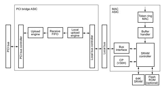
**Packet Upload** Any operation that the host performs on receive packets is performed on the top packet only. The top packet is the oldest packet in the FIFO, and the one that the upload DMA engine is either transferring or is ready to transfer next. It is also the packet for which status is made visible to the host.
