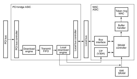
The download engine tries to keep the FIFO full until the end of a packet has been downloaded, while also observing rules on burst size and frequency that are designed to optimize transfers across the PCI bus.
