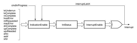
Enables have an immediate effect on indications and interrupts. If a particular interrupt is pending and the host clears its enable bit in the IndicationEnable register, the indication, though still pending, appears as a zero in the IntStatus register and no longer contributes to the assertion of the interrupt line on the host bus (although the interrupt line stays asserted because of the interruptLatch bit).
