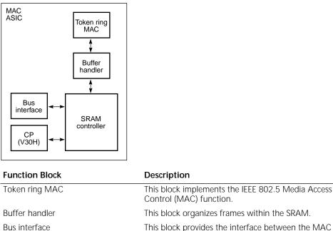
This block provides the interface between the MAC ASIC and the local bus. This block is the V30H communications processor. This block arbitrates among various requesters for
