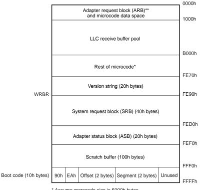
Figure 3 RAM-Based Configuration Memory Usage
