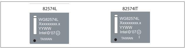
Figure 2. Production Top Marking Example With Identifying Marks
