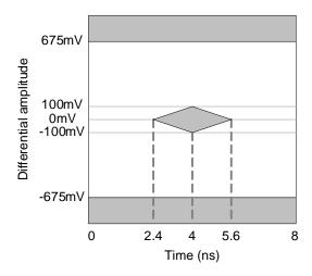
Figure 8. Kumeran (Serial) Receive Eye Diagram
