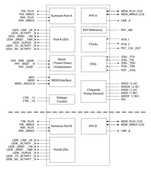
Figure 13. 82563EB/82564EB Interfaces
