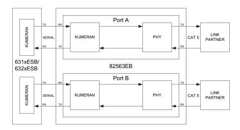
Figure 1. 82563EB Dual Port Block Diagram
