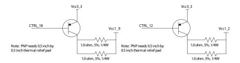
Figure 5. 82563EB 1.9V and 1.2V internal LVR schematic
