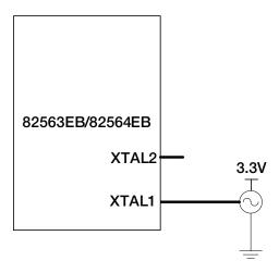
Figure 9. External Clock Oscillator Connectivity to 82563EB/82564EB
