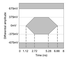
Figure 7. Kumeran (Serial) Transmit Eye Diagram
