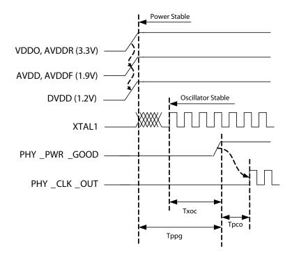
Figure 10. 82563EB/82564EB Reset Timing
