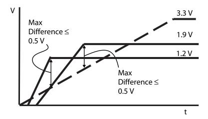
Figure 3. 82563EB/82564EB power up sequencing with external regulators
